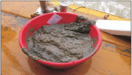
An example of a benthic grab sample before sieving.
